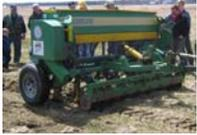
**AITCHISON DRILL 8' wide:** The Aitchison is a no-till drill made specifically for interseeding and complete renovation of pastures. It can handle a complete seed mix in one hopper and does a very good job in most situations, except it does not go through large amounts of long residue very well. Just a warning, **it will pull up some stones if they are near the surface.**
